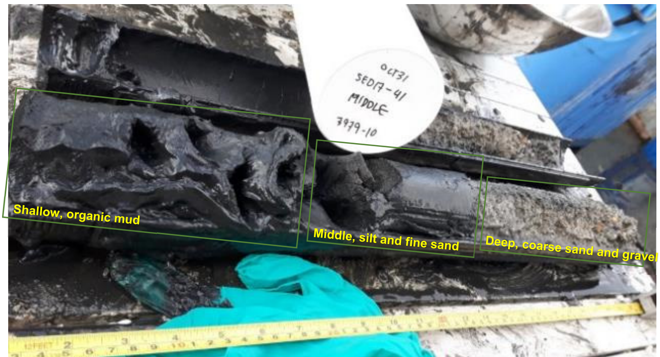
Figure 2: Core sample from location SED17-38 showing the three different sediment classifications
