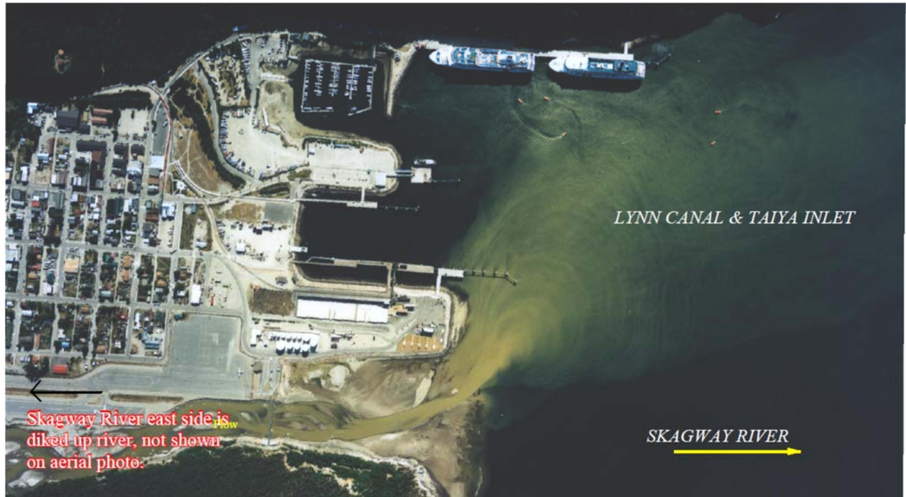
Figure 15: May 21, 2004 aerial photo of the Skagway River mouth and sediment plume (USACE 2008).
