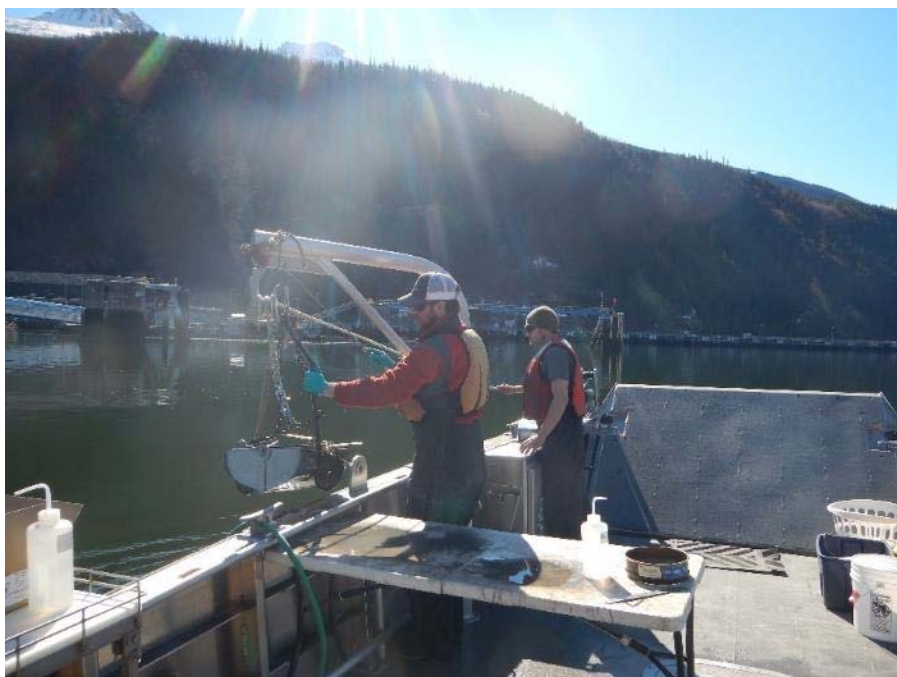
Photo 7: Depiction of Work Area and Van Veen Sampler in Use
