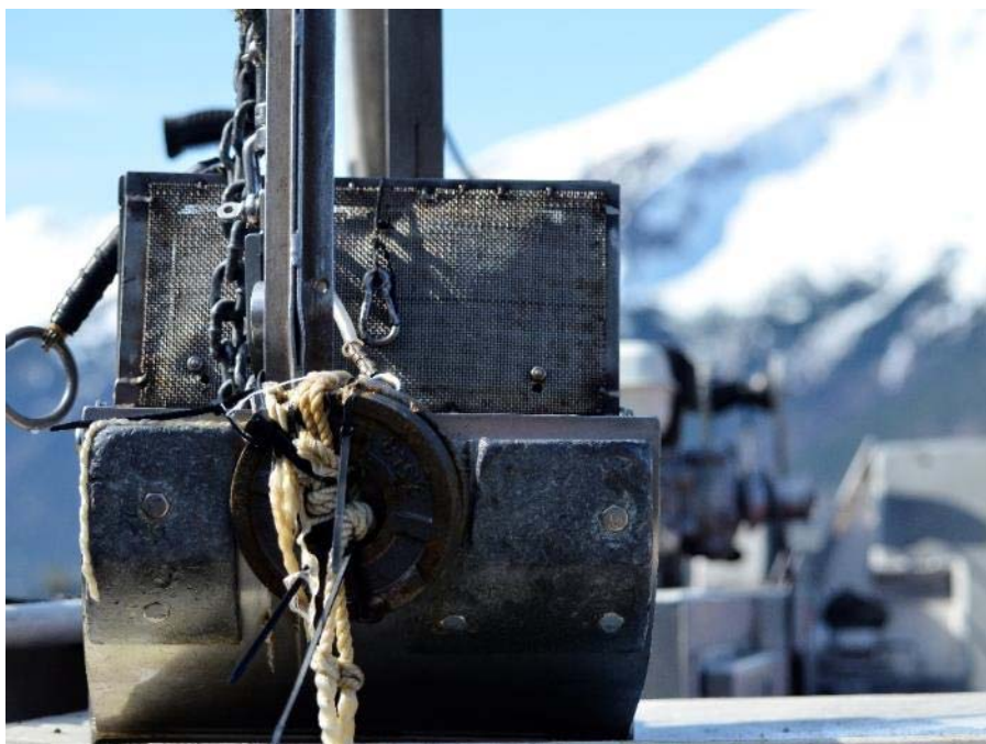
Photo 10: Depiction of Additional Weight Added to Van Veen.
