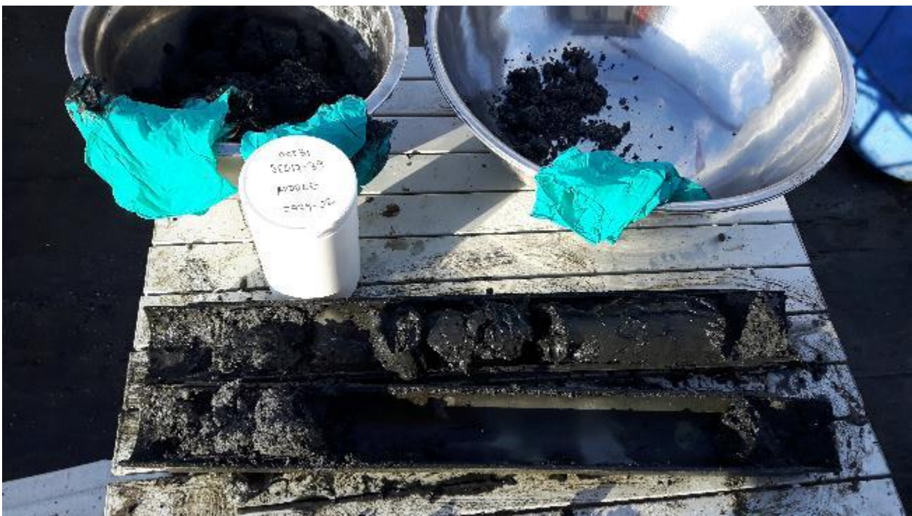
Photo 12: Sample location SED17-34, core recovered in the 3rd spoon
