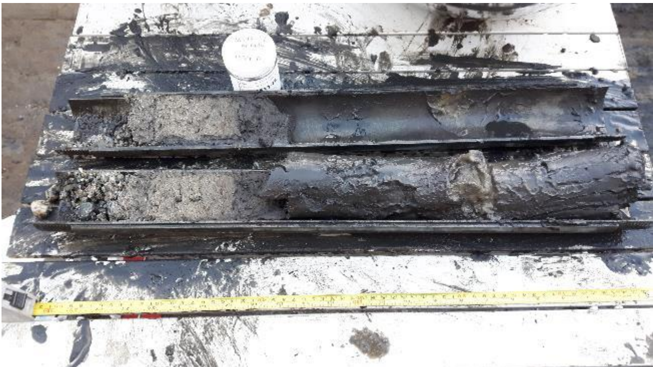
Photo 18: Sample location SED17-37, core recovered in the 4th spoon.
